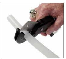
1. Cut tube at 90-degrees. Do not crush outside diameter of tubing with cutters. To achieve a clean cut, slightly rotate cutter during blade engagement.
