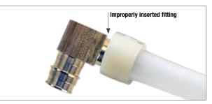
Fitting not inserted completely into expanded tube and ring. Ring not fully covering WaterPEXa tubing.
