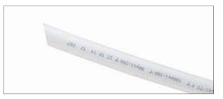
Tube not cut squarely - ring and tube need to be mated perfectly and installed fully over F1960 barb for a viable seal.
