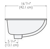
A.D.A. Lavatory Installation Requirements: Lavatories shall be mounted with rim/ counter surface no higher than 34 inches (86.4 cm) above finished floor. Provide a clearance range of 27-29 inches (68.6 - 73.7 cm) from the floor to the lavatory bottom or lavatory apron depending upon de type installed. For complete details on installation requirements, see A.D.A. Installation Handbook.
