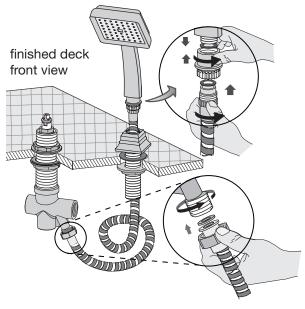
Step 6 Install plping and check for leaks
