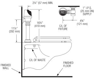
When installing the Sloan ECOS® Electronic in a handicap stall: Per the ADA Guidelines (section 604.9.4) it is recommended that the grab bars be split or shifted to the wide side of the stall.
