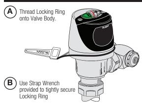
Important: The Locking Ring must be installed down past the valve body threads by at least one thread. If difficulty is experienced installing the Locking Ring, turn the Locking Ring back and forth, each time working it further down the threads. The Locking Ring will act as a thread chaser in the event there has been a build-up of matter on the threads of the old valve body.
