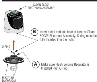
Push Diaphragm securely against underside of Sloan ECOS® Electronic Assembly. Place entire Assembly onto the Valve Body.
