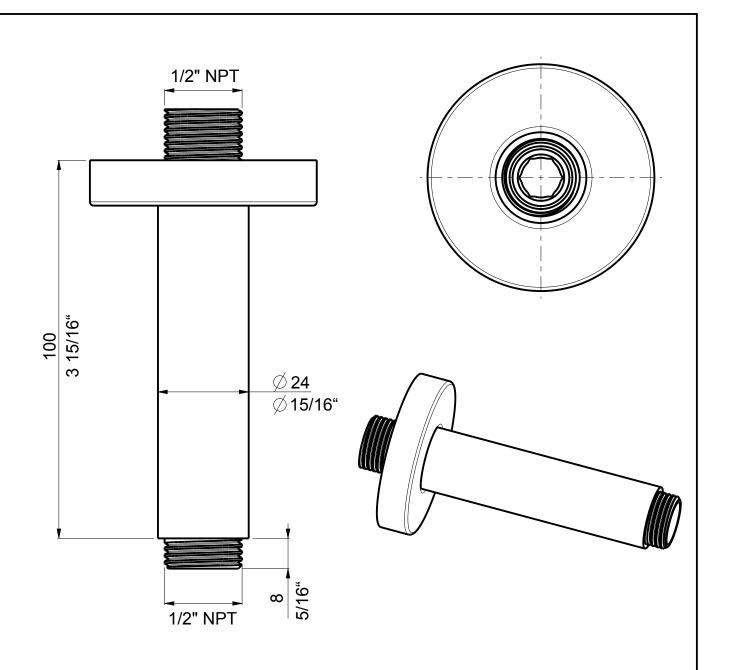
Note: Please apply thread seal tape (also known as plumber's tape) to all threads
