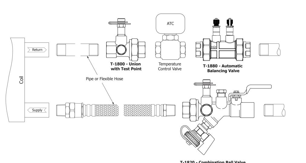
T-1820 - Combination Ball Valve with Strainer, Drain and Test Point
