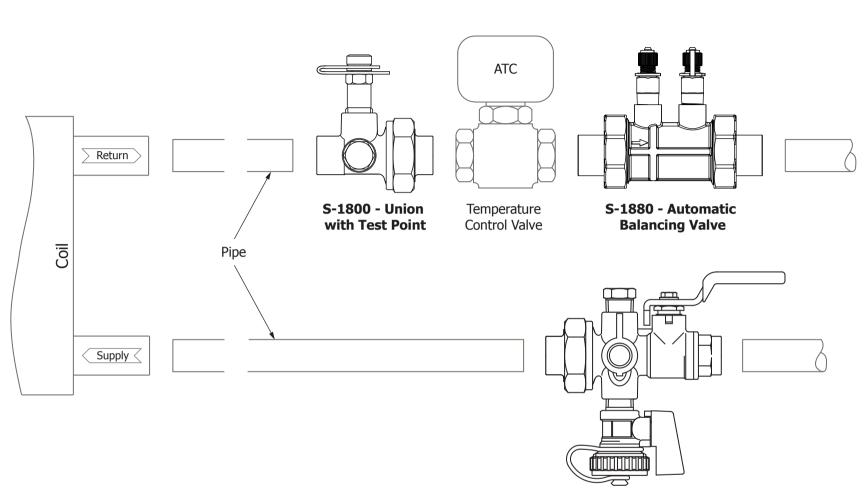
S-1830 - Combination Ball Valve with Drain and Test Point
