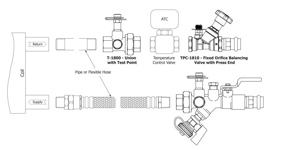
PCT-1820 - Combination Ball Valve with Strainer, Drain and Test Point with Press End
