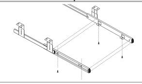
Align the shelf 1/16" shorter than the slide plastic protector. Fasten shelf with (4) recommended #8 x 5/8" pan head wood screws
