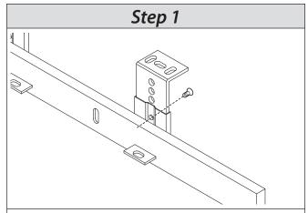
Place L-shaped mounting brackets for ideal height and direction. Fasten with M4 x 5 pan head machine screws
