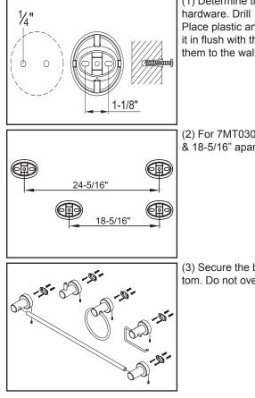
(1) Determine the installation location for the bathroom hardware. Drill 1/4" diameter hole approximate 1-1/8" apart. Place plastic anchors into the drilled holes, use hammer to tap it in flush with the wall. Place the mounting plate and secure them to the wall with the help of mounting screws.
