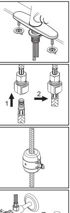
(3b) Thread and tighten both mounting nuts to mounting bolts from underneath the sink to secure faucet on the sink.
