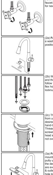
(1) Shut off the water supply. Remove old faucet. Clean mounting surface in preparation for new faucet
